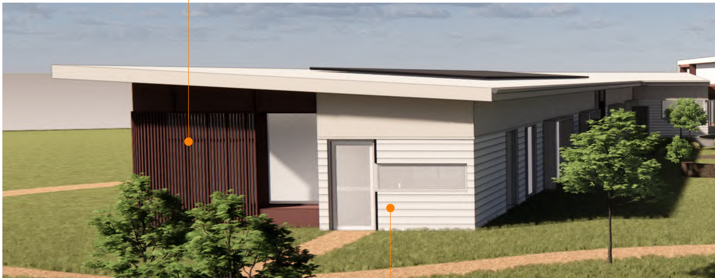
FIBRE CEMENT CLADDING WITH COLOURED PAINT FINISH AND COVER BATTENS (FC02) COLOUR DEEP NEUTRAL. NOTE: COLOUR SHOWN INDICATIVE.
